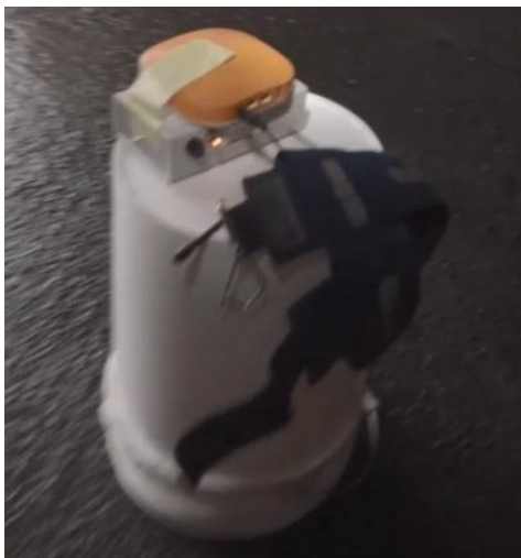
2 nd node design as used at Russell Vale for final testing in March 2017 (note: positioned on top of a bucket, has independent large battery pack underneath node, and blue CSE pouch adjacent to node positioned to give perspective)
